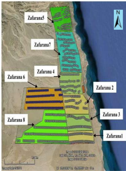
Figure 3. The Distribution of 698 Borings at Zafarana wind farms
