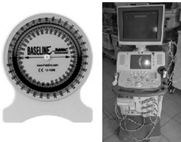
Fig. (1): Instruments; (A): Baseline bubble inclinometer. The blue color is the moving fluid within the inclinometer, (B): Diagnostic ultrasound equipment.
