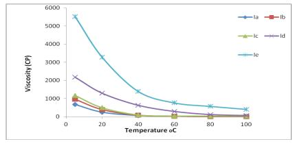
Fig. 10. Relation between viscosity (CP) and temperature (oC) for ILs (Ia-Ie).
