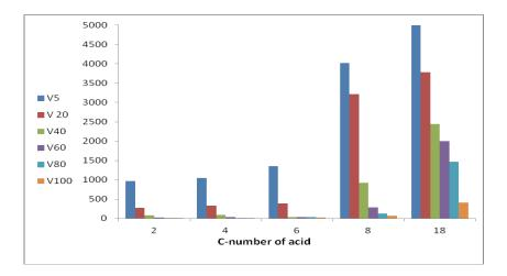
Fig. 15. Relation between viscosity (CP) and C-number of acid at temperature for ILs (Ia-Ie).
