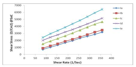
Fig.12. Relation between shear stress and shear rate at low temperature for ILs (Ia-Ie).
