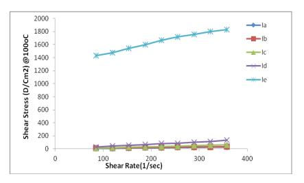
Fig. 14. Relation between shear stress and shear rate at low temperature for ILs (Ia-Ie).
