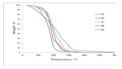
Fig. 8. Thermal gravimetric analysis for the prepared ILs (Ia-Ie).
