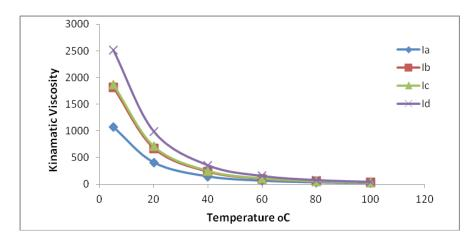
Fig. 9. Relation between kinematic viscosity and temperature.
