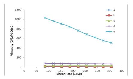
Fig. 13. Relation between viscosity (CP) and shear rate at high temperature for ILs (Ia-Ie).
