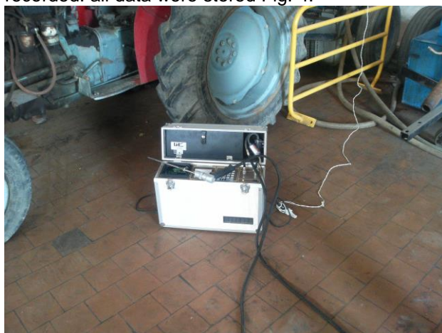
Fig. 4: The exhaust gas analyzer
