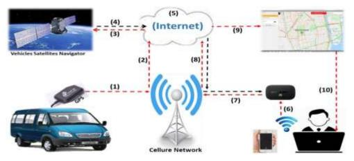
Figure No. (7): Car Tracking System Architecture
