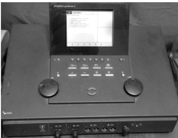
Fig. (3): Electrotherapy device generating interferential current.
