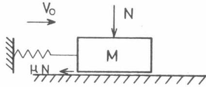
FIG. 1 Simple elastic rubbing system
