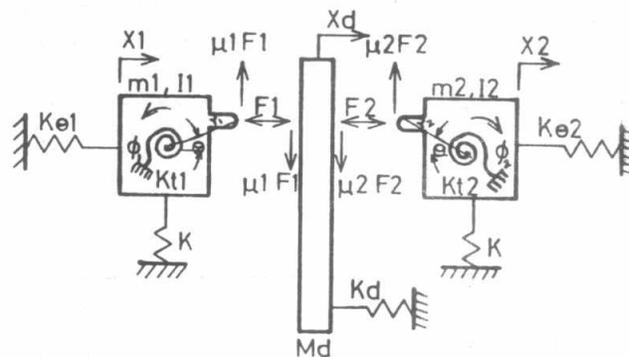
FIG. 7 Dynamic model of disc brake assembly
