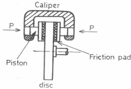
FIG. 6 Basic features of a real disc brake assembly
