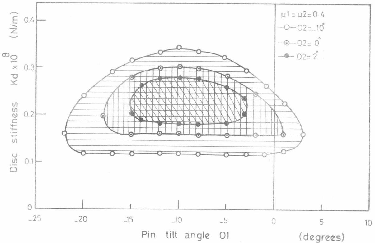
FIG. 9 Instability regions for the disc brake at moderate friction coefficients
