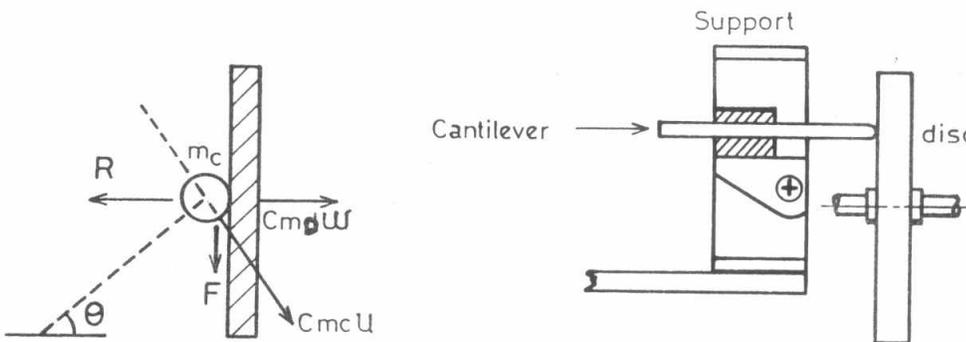
FIG. 3 Disc-Cantilever model
