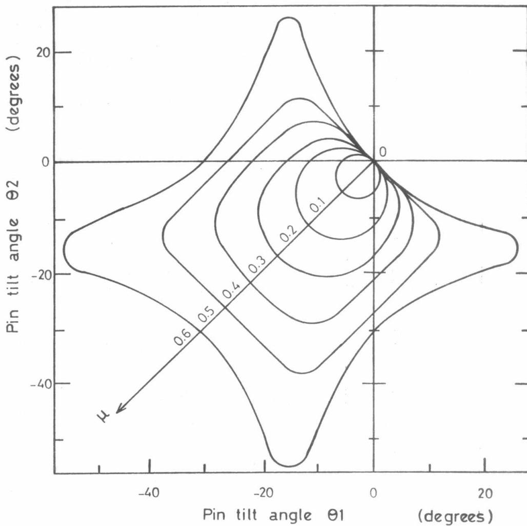
FIG. 10 Instability regions for the disc brake at different coefficients of friction
