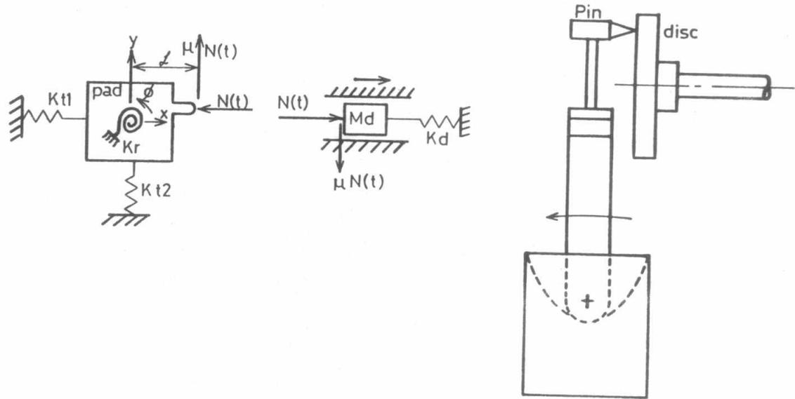
FIG. 5 Four degree of freedom pin-disc model
