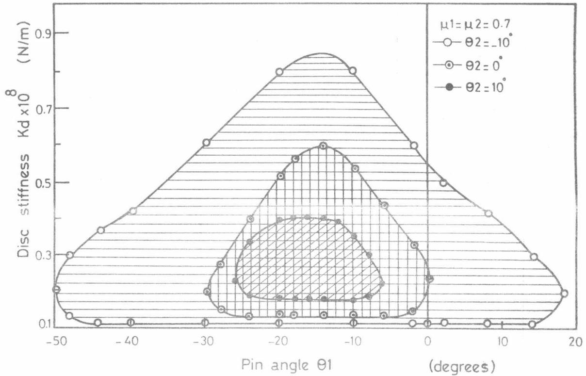
FIG. 8 Instability regions of the disc brake at high friction coefficients
