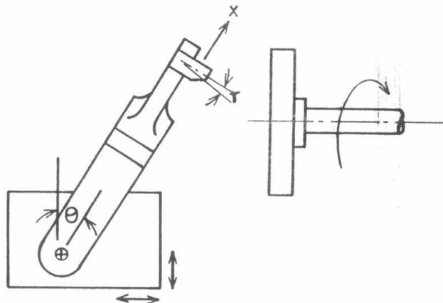
FIG. 4 Pin-disc model (8)
