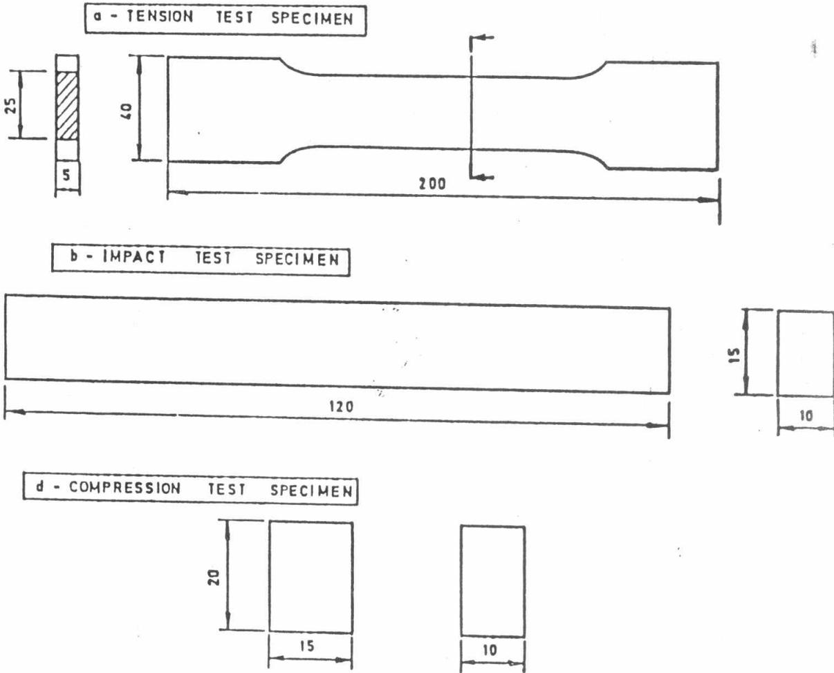
FIG. 1 - MECHANICAL PROPERTIES TEST SPECIMEN
