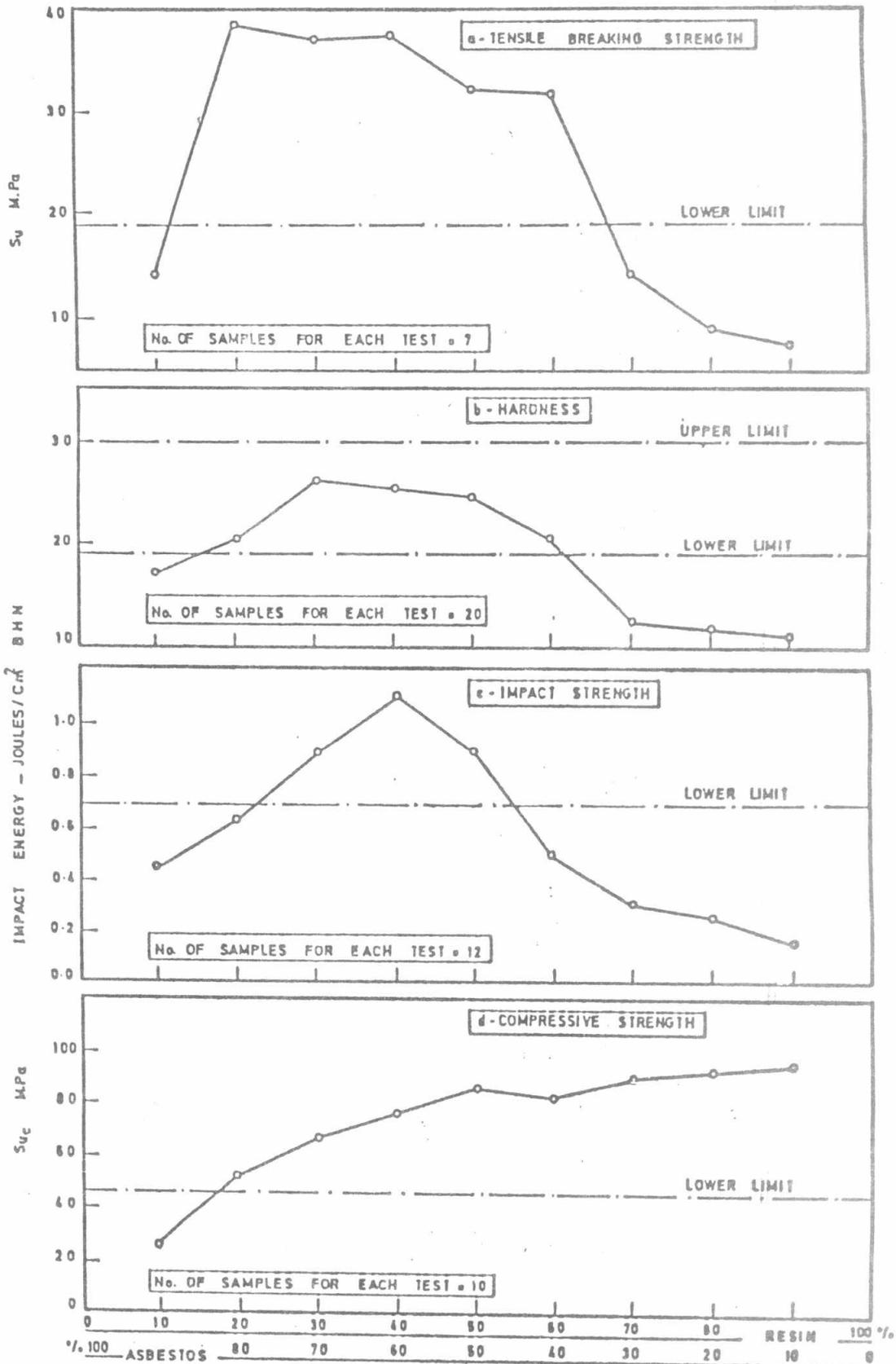
FIG. 2 - EFFECT OF RESIN / ASBESTOS CONTENT ON MECHANICAL PROPERTIES OF ASBESTOS FILLED RESIN FRICTION COMPOUND
