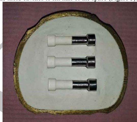
Figure 3: The surface treated alloy specimens placed in the mold cavities.
