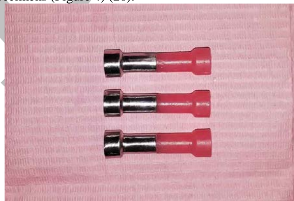
Figure 4: Heat cured PMMA-alloy specimens.
