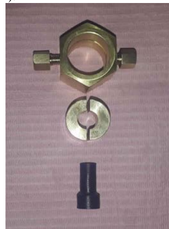
Figure 2: Wax pattern corresponding to half of the tensile bar specimen and the split copper mold.
