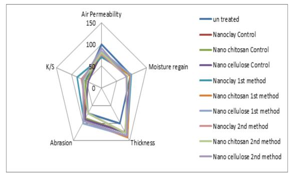
Fig. 4: Radar chart of treated viscose fabrics dyed with direct dyes
