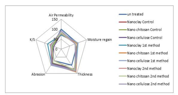
Fig. 5: Radar chart of treated viscose fabrics dyed with reactive dyes
