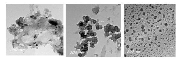
Fig. 2 (a, b, c):TEM micrograph of the nano materials used in the treatment of viscose fabrics<br/>a) nanochitosanb) nanoclayc) nanocellulose
