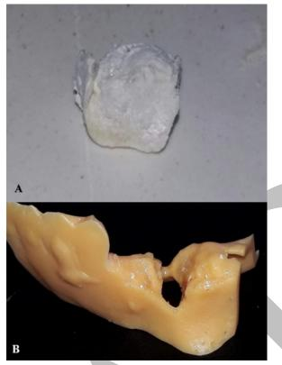
Figure (1): Zirconia porous scaffold
