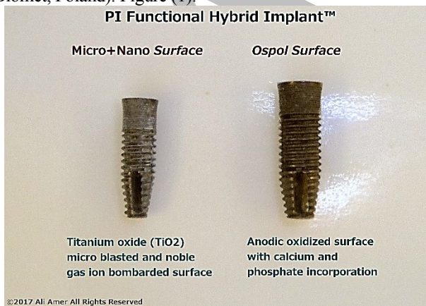
Figure 1: Photograph showing the P-I Functional Hybrid implant with the two surface treatments.
