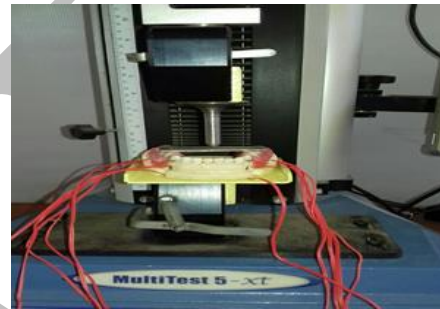
Figure (2): study model under central loading
