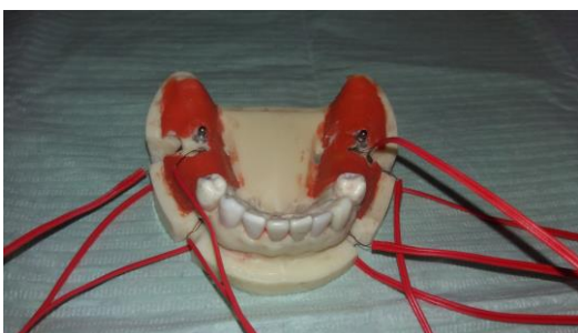
Figure (1): Epoxy resin model with strain gauges sensors.
