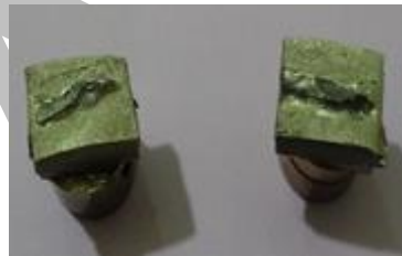
Figure (2): Specimens coated with Gold-Palladium.
