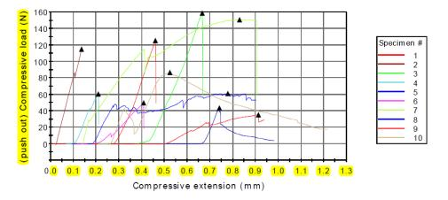
Fig. 2. Maximum load applied on the samples exposed to radiation (N).
