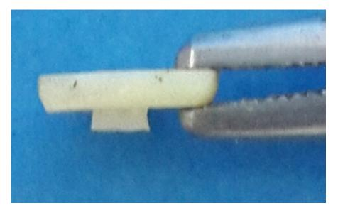
Fig. 1. The failure reported on extrusion of the restoration from the prepared specimen.
