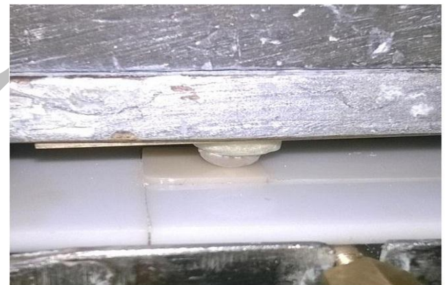
Fig. 2: Antagonist enamel cusp occluding flat ceramic specimen.
