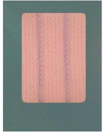
Fig 2: Proceed® mesh (polypropylene soft mesh encapsulated with PDS and layered in one side by ORC)
