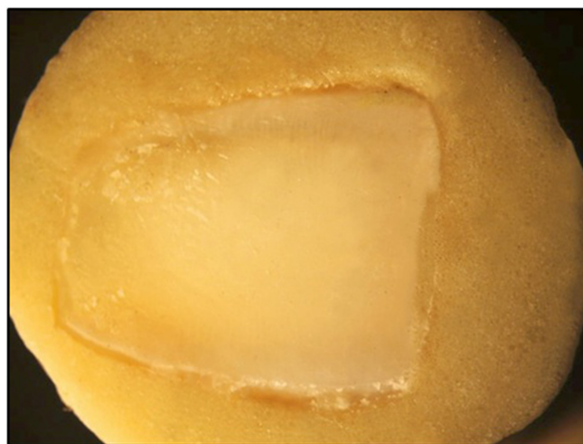
Fig. (4): Adhesive failure in Group A (antioxidant treatment).
