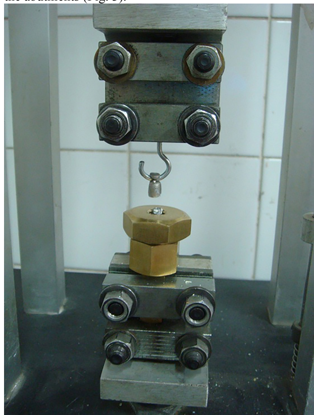
Figure 3: coping dislodged from the abutment – universal testing machine
