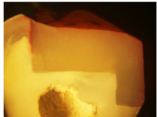
Figure 3: Sectioned specimens with microleakage score 3 (dye penetrates into the dentin) at: Occlusal wall.
