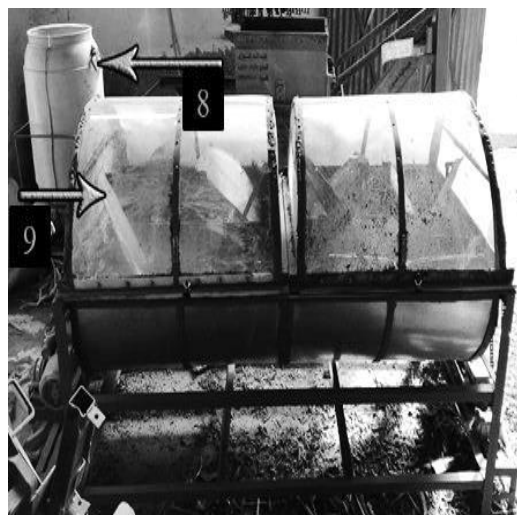
1-The gate of vessel. 2-Transmission gear. 3-Frame. 4-Gear box. 5-The control unit. 6- reverse movement unit. 7- The motor. 8- water tank. 9- Impeller.
