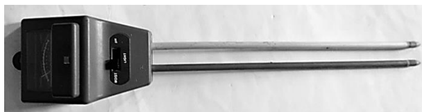
Fig.5. Moisture content and pH measuring device.
