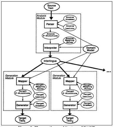
Figure 9: The run-time architecture of KANT
