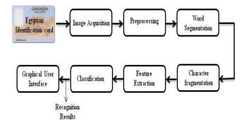
Figure 5: The Proposed Arabic OCR Block Diagram
