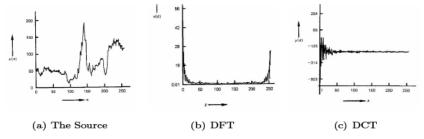
Figure 8: Energy distributions in different transforms
