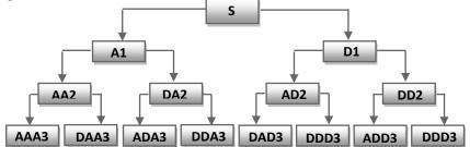
Figure 7: Signal decomposition using wavelet packets [15].
