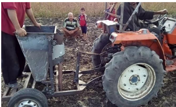
Fig. 2A. The planter prototype mounted on the tractor.
