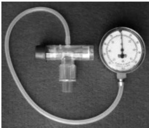
Fig. (1): Respiratory pressure Gauge with maximum effort indicator.
