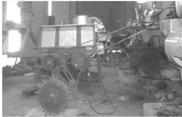
Fig. 3. The transmission unit was provided with a lathe as a source of power
