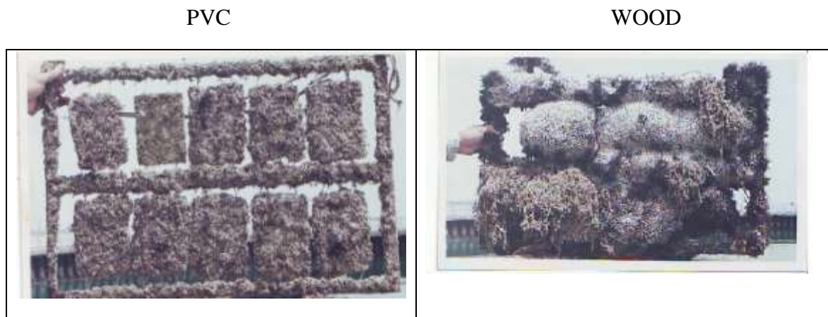
Fig. (2). Fouling organisms accumulated on PVC (1) and wood panel at the inlet of seawater at the entrance of Attaka power station during 2006.
