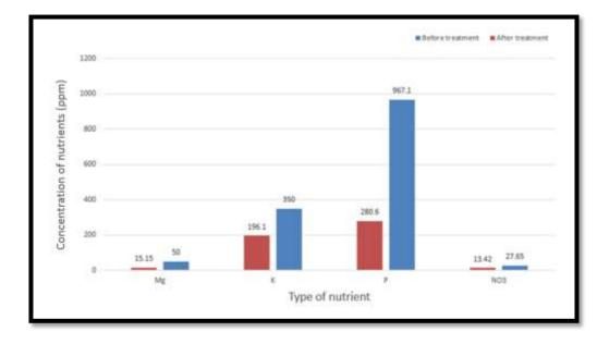
Fig..3. Removal efficiency of nutrients by C. vulgaris from 100% wastewater.
