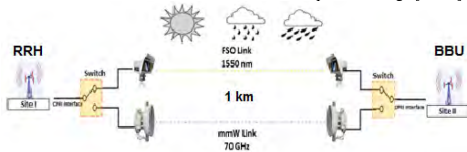
Fig.4: Simulated network topology connected RRH with BBU pool.
