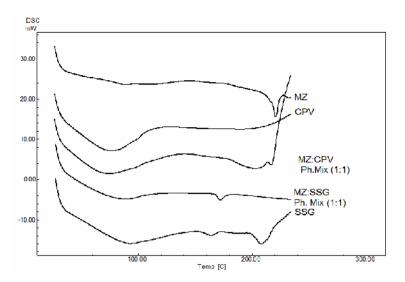
Fig. 1a: DSC thermograms of MZ HCl alone, SSG alone, CPV alone and their physical mixtures (1:1).
