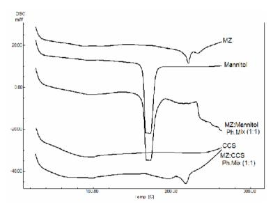
Fig. 1b: DSC thermograms of MZ HCl alone, CCS alone, Mannitol alone and their physical mixtures (1:1).
