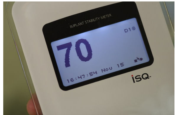
Figure 4: A photograph showing Ostell reading after one and half month (secondary stability).
