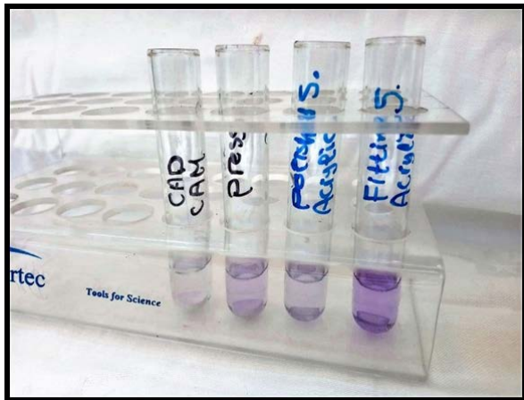
Figure (5): Showing different acetic acid elution color owing to different stain uptake, corresponding to different amounts of biofilm formation.
