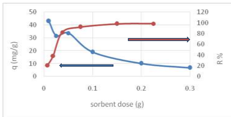
Fig. 12. Effect of adsorbent dosage of silica/corn cob nanocomposite on removal efficiency and the uptake of methylene blue (pH=7.5).
