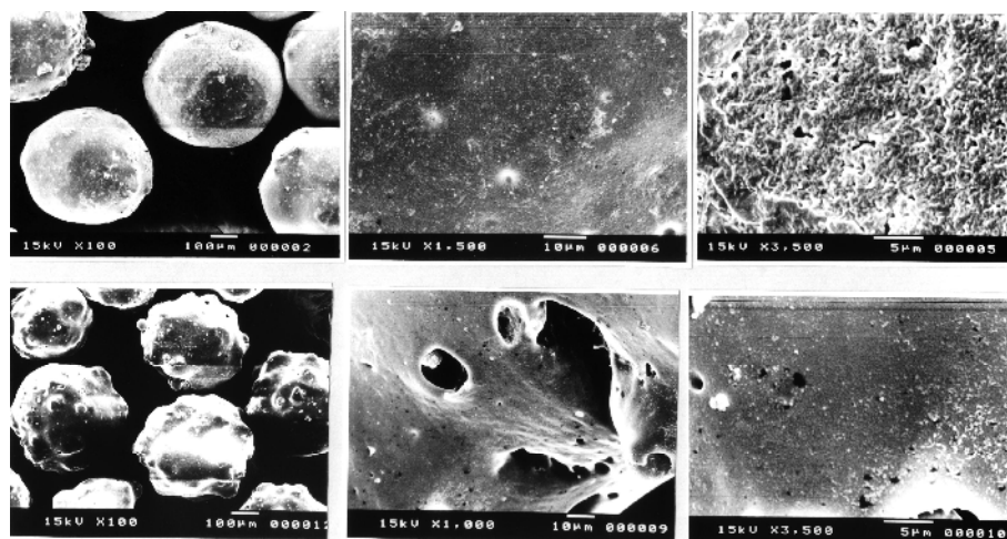
Fig. 5: Representative scanning electron micrographs of Nefopam HCl-loaded CAB microcapsules prepared at core : coat ratios of (A) 1:2 and (B) 1:1.
