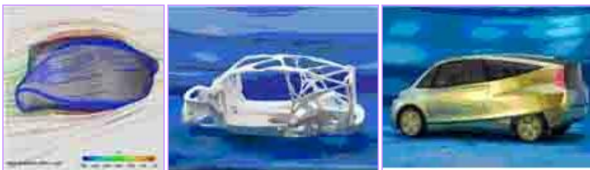
Fig. 9. Daimler Chrysler bionic car inspired by the box fish and tree growth patterns.
