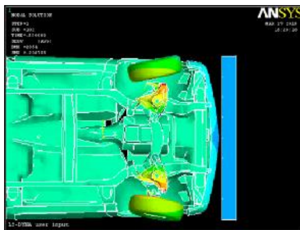
Fig. 7. The bottom view of the frontal crash test under low speed of 5 miles/hour. Crash at time = .15000 sec.
