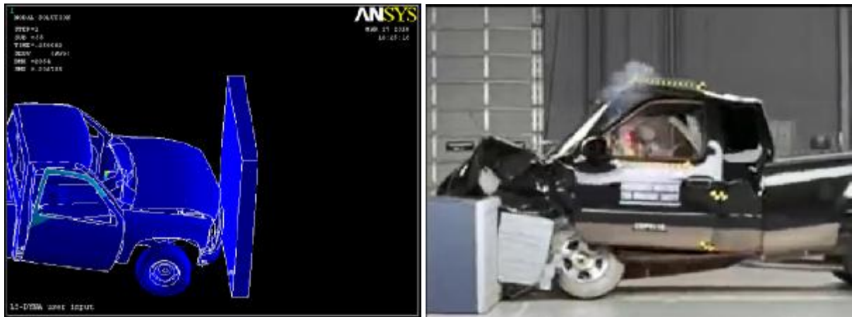
Fig. 9. The frontal crash at speed of 35 miles/hour. Left FE model. Right the IIHS test. Time = 0.07500 sec.
