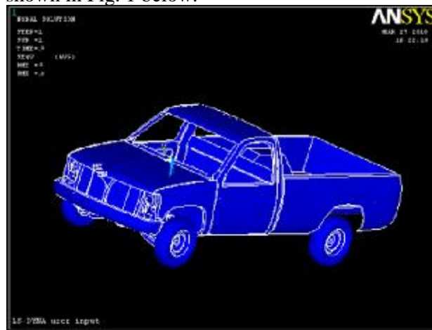
Fig. 1. The structure of the Imported NHTSA model of the Ford Truck to ANSYS LS-DYAN System.
