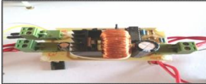
Fig.4: Executed buck converter after printing and assembling.
