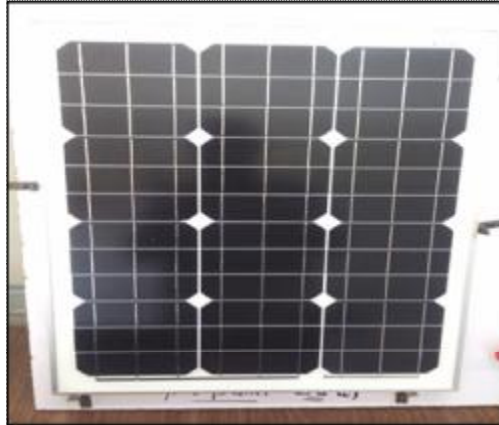
Fig.5: 50W MONO solar panel.
