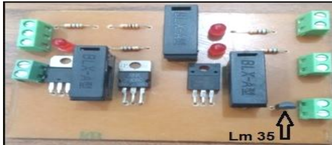
Fig.8: LM 35 temperature sensor in input and output printed circuit board.
