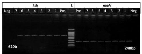
**Fig. (2):** Agarose gel electrophoresis of amplified tsh PCR product (620bp) and amplified eaeA PCR product (248bp).
