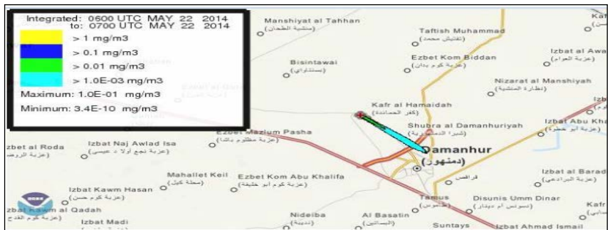
Fig. (44): Dispersion Model for CO emission from Damanhur Power Plant during spring
