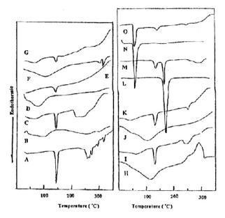
Fig. 2: DSC thermograms of Verapamil (A); CP974P (B); physical mixture (1:1) of VH and CP974P (C); HPMC (D); physical mixture (1:1) of VH and HPMC (E); NaCMC (F); physical mixture (1:1) VH and NaCMC (G); sodium alginate (H); physical mixture (1:1) of VH and sodium alginate (I); guar gum (J); physical mixture (1:1) of VH and guar gum (K); mannitol (L); physical mixture (1:1) of VH and mannitol (M); PEG6000 (N); physical mixture (1:1) of VH and PEG6000 (O).
