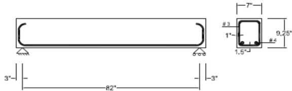
Figure (13): Details of beam specimens [9].
