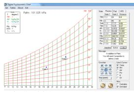
Fig. (4). Digital Pyschrometric chart program
