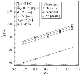
Fig. (16). Rejected heat versus water/air mass flow ratio (MR) with and without packing
