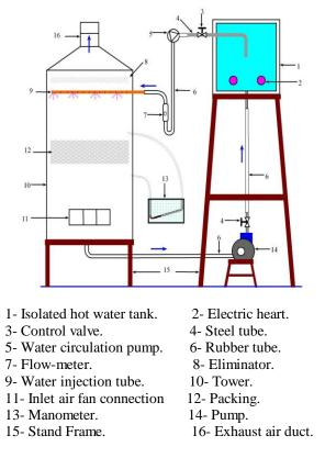
Fig. (1). Experimental apparatus details
