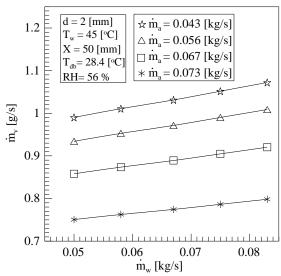
Fig. (8). Effect of water mass flow rate on the vaporization for different air mass flow rate.
