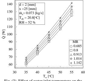
Fig. (3). Effect of water inlet temperature on the rejected heat for different mass flow rate ratio.
