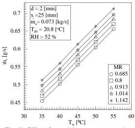
Fig. (5). Effect of water inlet temperature on the vaporization rate for different mass flow rate ratio.
