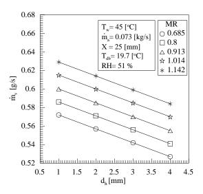
Fig. (11). Effect of injection holes diameter on the vaporization rate for different mass flow rate ratio.
