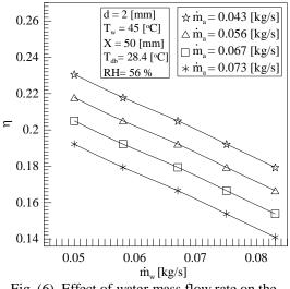
Fig. (6). Effect of water mass flow rate on the cooling tower efficiency for different air mass flow rate.
