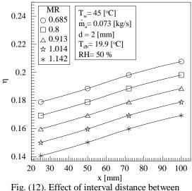
injection holes on the cooling tower efficiency for different mass flow rate ratio.
