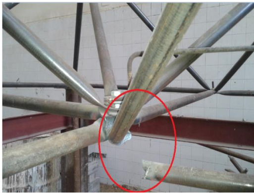
Figure 39: Collapsed members from the second test of truss#2
