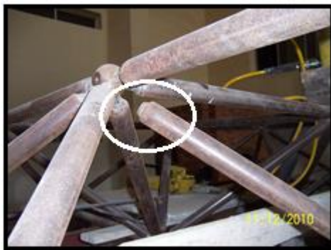
Figure 28: Collapse in connections (20&23) from the third test of truss#1
