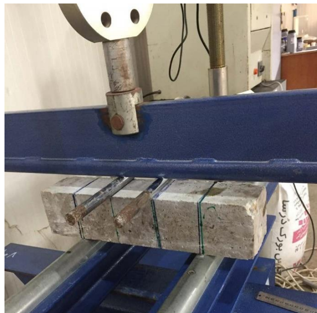
Figure 5: Modulus of Rupture Test
