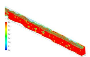
**Figure.14** Gas volume fraction in discharge passage for GLR 0.8%., at 0.0236 s.
