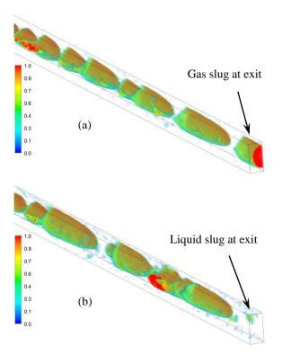
**Figure.6** Gas volume fraction in discharge passage at GLR 0.08%. (a) at 0.0565 s., (b) at 0.0584 s.
