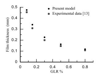
Figure.4 Comparison between calculated liquid film thickness and experimental
