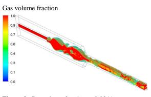
Figure.9 Gas volume fraction at 0.0341 s. and GLR = 0.5%.
