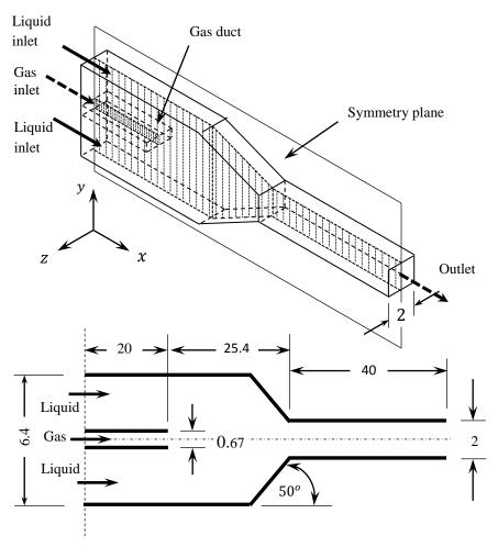
Figure 1. Details of effervescent atomizer model used in present work (dim. in mm)
