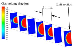
**Figure.7** Gas volume fraction contours for GLR= 0.08%. at 0.0565 s.
