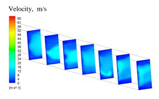
Figure.12 Mixture velocity contours for GLR=0.5%, at 0.0341 s.
