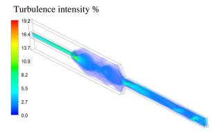
Figure.11 Mixture turbulent intensity contours for GLR=0.5%, at 0.0341 s.
