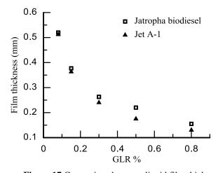
Figure.17 Comparison between liquid film thickness for Jatropha biofuel and Jet-A1 aviation fuel.
