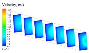
Figure.8 Mixture velocity contours. GLR= 0.08% at 0.0565 s.
