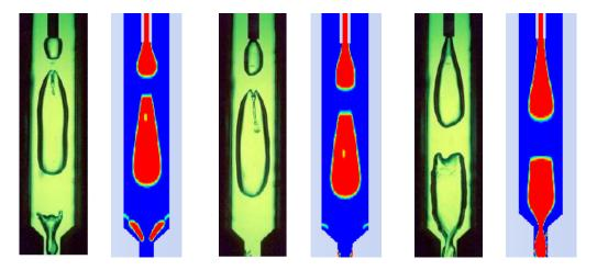
Figure.3 Comparison between gas void fraction simulation results and experimental photo for GLR=0.08% and QL=0.38 L/min [13].
