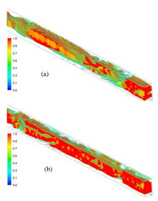
**Figure.10** Gas volume fraction in discharge passage for GLR 0.5%. (a) at 0.0341 s., (b) at 0.0240 s.
