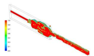
**Figure.13** Gas volume fraction in discharge passage for GLR 0.8%, at 0.0236 s.
