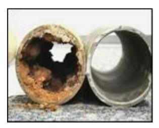
Fig 12: sediments in pipes
