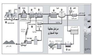
Fig(1): Wastewater treatment stages applied in Centralized system in Egypt - www.hcww.com.eg
