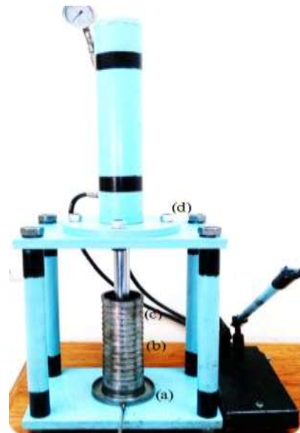
(a) L Housing (c) Circular plates (d) Hydraulic press Figure 4: Hydraulic press components.
