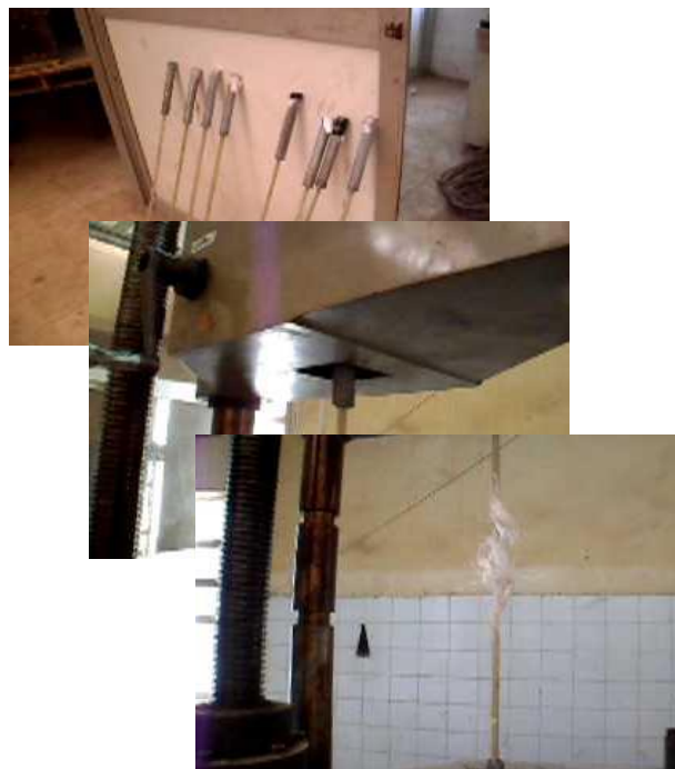
Fig. (3) Experimental setup for GFRP specimens
