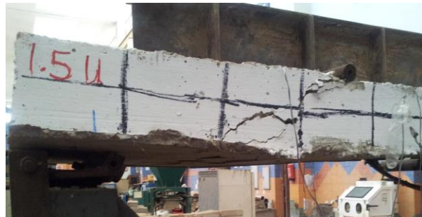
Fig. (6) Failure mode of slab S1-1.5U
