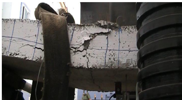
Fig. (7) Failure mode of slab S6-2O
