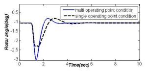
Fig.9Rotor angle for single and multi operating conditions
