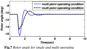
Fig.7 Rotor angle for single and multi operatin conditions
