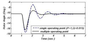
Fig. 11 A comparison between single and multiple design response for rotor angle
