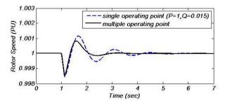
Fig. 10 Acomparison between single and multiple design response for rotor speed
