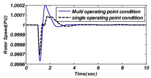
Fig.8Rotor speed for single and multi operating conditions
