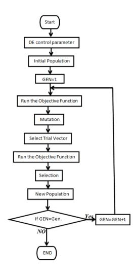
Fig. 1 flow chart of Differential Evolution technique
