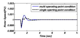
Fig. 6 Rotor speed for single and multi operating conditions
