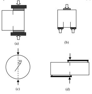
Fig. 1 Mode II fracture toughness test geometries
