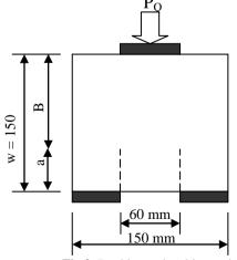
Fig.3 Double notch cubic specimen
