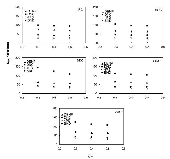
Fig.7 Notch depth to specimen width ratio (a/w) versus mode II fracture toughness K<sub>IIc</sub> for different concretes.
