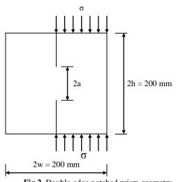
Fig.2 Double-edge notched prism geometry.
