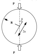
Fig.5 Cracked Brazilian disc specimen
