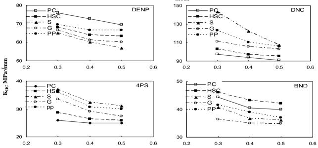
Fig.6 Notch depth to specimen width ratio (a/w) versus mode II fracture toughness K<sub>IIc</sub> for various test setups.
